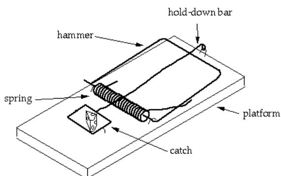
A simple mouse trap is made from at least six components: the platform, the spring, the hammer, the catch, the holdback bar, and staples. Without any of the components the machine will not function. Furthermore, each of the components have to be designed to a specific size and placed in a specific place in order for the mouse trap to function.
